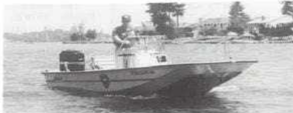
The 17-foot Boston Whaler is powered by a 100 HP outboard.
